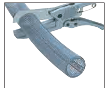
Cutting of nylon hoses
